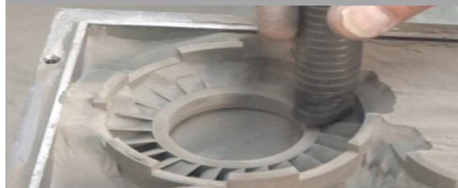
Depowdering reveals the 3D Metal Printed part
