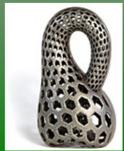
Post sintering, the metal particles are metallurgically bonded into a high strength finished part
