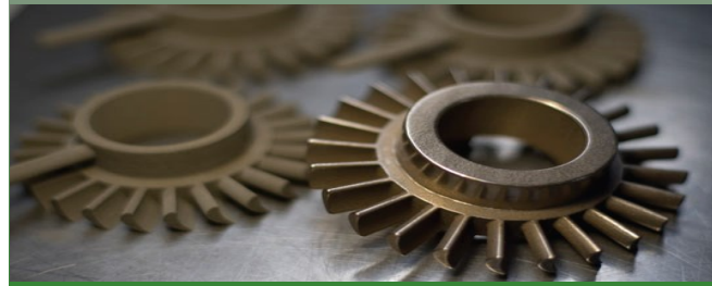
Post sintering, the metal particles are metallurgically bonded into a high strength finished part
